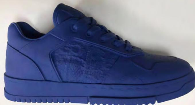
We used our expertise in 3d scanning to capture Dior's latest collection of Hitops in 3d. The resulting scans were then cleaned and embellished. Once we were happy with the scans they were then 3d printed. The hitops were then moulded and cast in various different finishes and pantone colours.
